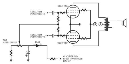
the small electrolytic capacitor smooths problematic ripple from the signal,
