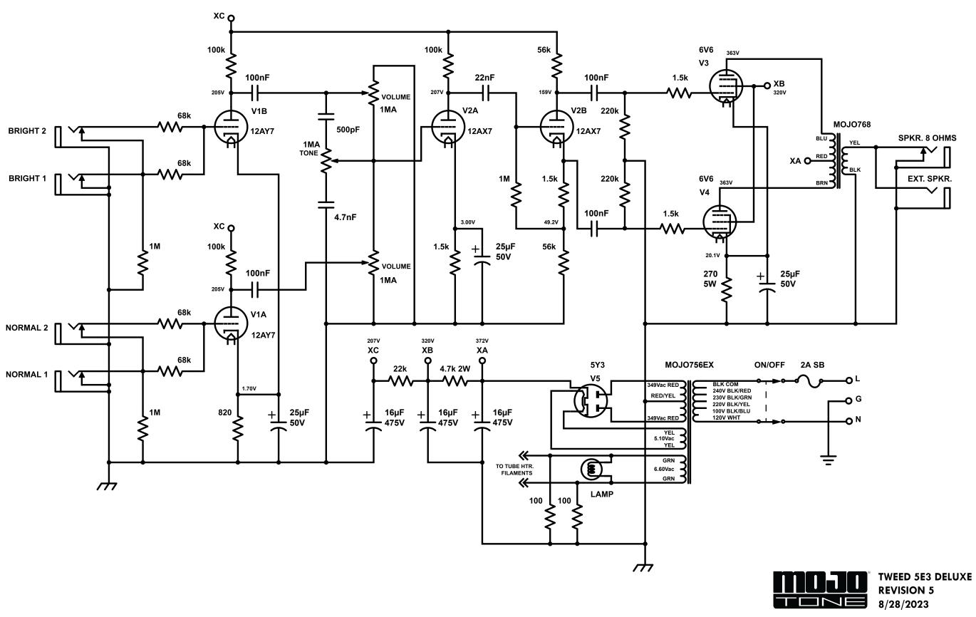
All resistors are rated for 1/2W unless specified.
